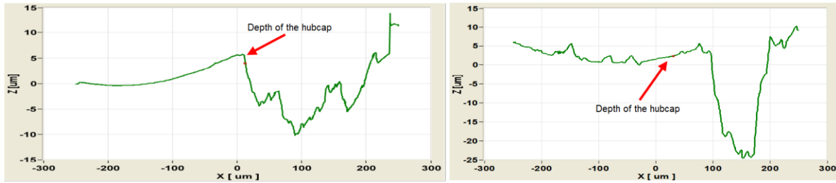
Figure 6. 2D profile of the worn region of the fly ash samples region with more accentuated wear and formation of valleys.
